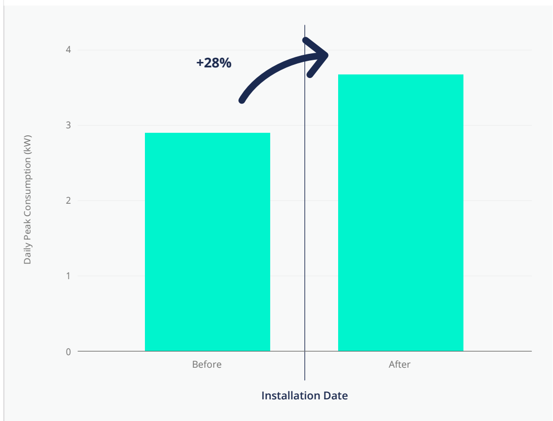
FIGURE 3 Average daily peaks (kW) for a household before and after installing a charging solution
